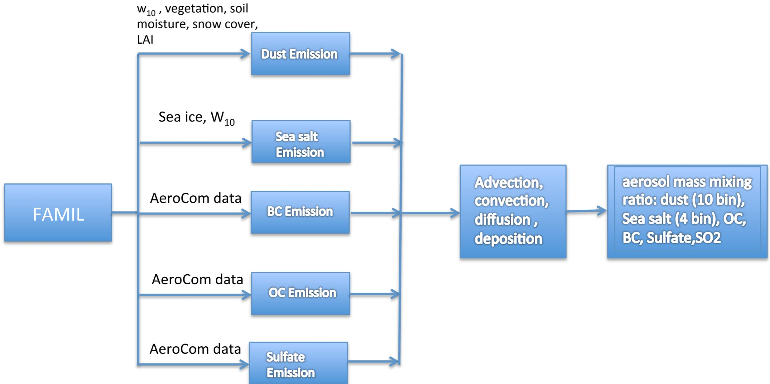
Structure of aerosol processes including emission, transport, and deposition in FAMIL
