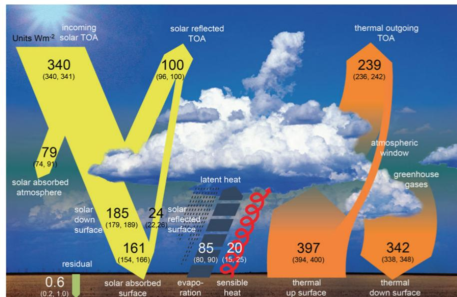
**Fig. 1** Schematic diagram of the global mean energy balance of the Earth. Numbers indicate best estimates for the magnitudes of the globally averaged energy balance components together with their uncertainty ranges, representing present day climate conditions beginning of the twenty first century. Estimates and uncertainty ranges based on discussion in Sect. 5. Units  $\text{W m}^{-2}$
